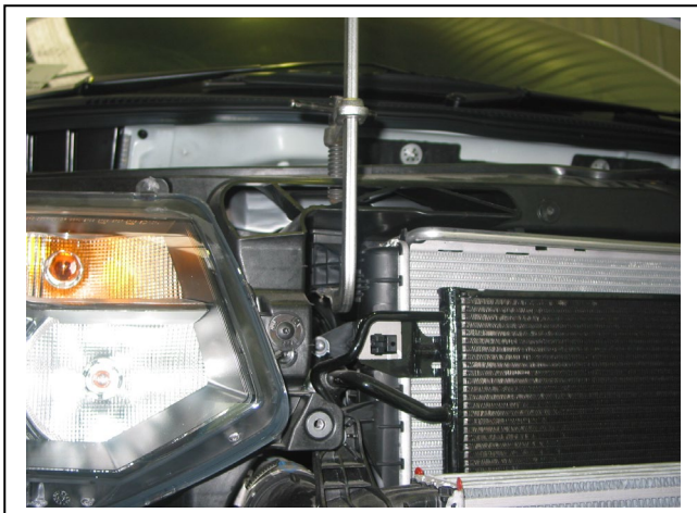
Figure 5: Supporting radiators using sliding “c” clamps under top mount. Note position of clamp
