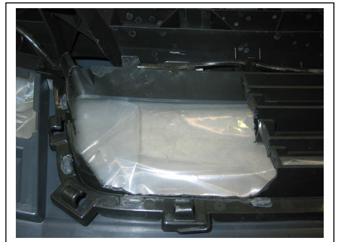
Figure 12: Remove outer sections centre grille. Remove lower section to house top mount.
