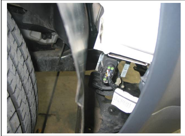
Figure 3: Wiring harness to be disconnected. Harness is removed with plastic bumper.
