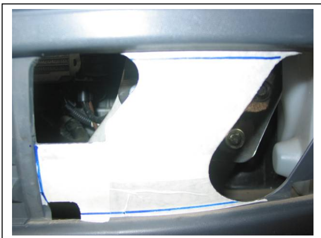
Figure 11: Remove marked section from plastic bumper cover.
